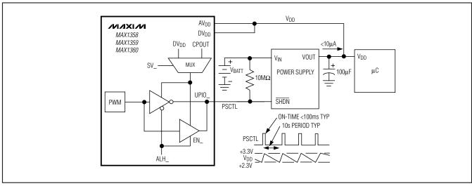
Figure 35. Power-Supply Sleep-Mode Duty-Cycle Control
