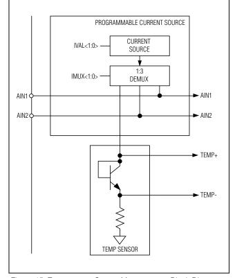
Figure 15. Temperature-Sensor Measurement Block Diagram
