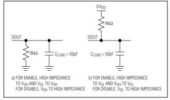
Figure 2. DOUT Enable and Disable Time Load Circuits
