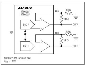
Figure 25. DAC Unipolar Rail-to-Rail Output Circuit
