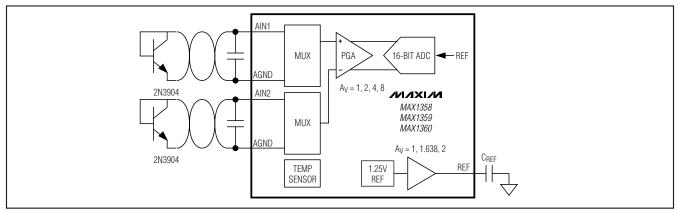
Figure 30. Temperature Measurement with Two Remote Sensors
