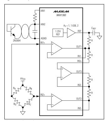
Figure 31. Strain-Gauge Measurement with Remote Temperature Sensor
