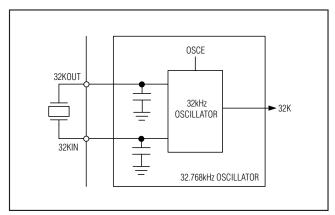
Figure 11. 32kHz Crystal-Oscillator Block Diagram
