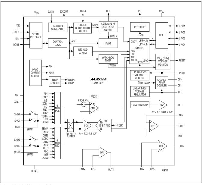
Figure 5. MAX1360 Functional Diagram
