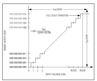
Figure 22. ADC Unipolar Transfer Function
