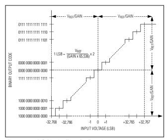
Figure 23. ADC Bipolar Transfer Function
