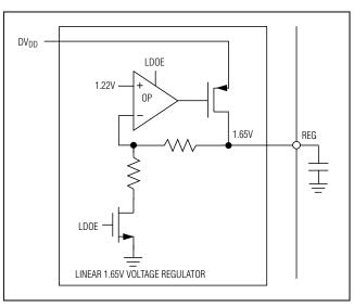
Figure 7. Linear-Regulator Block Diagram
