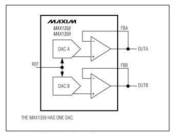
Figure 24. DAC Unipolar Output Circuit
