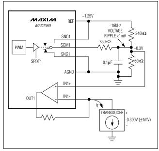
Figure 34. Sensor-Bias Voltage Trim Application
