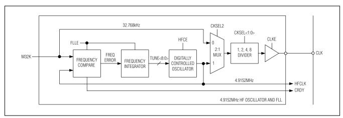
Figure 14. High-Frequency Clock and FLL Block Diagram
