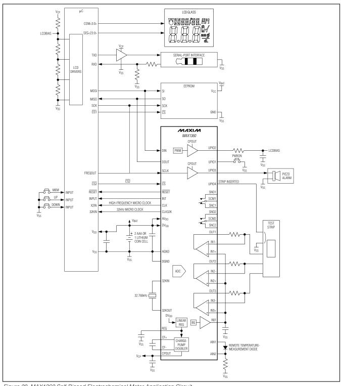
Figure 28. MAX1360 Self-Biased Electrochemical Meter Application Circuit
