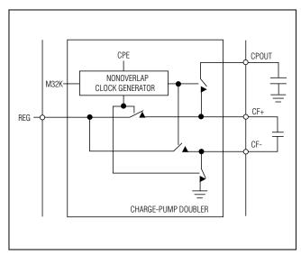
Figure 8. Charge-Pump Block Diagram
