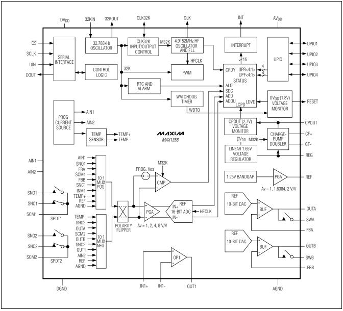
Figure 3. MAX1358 Functional Diagram
