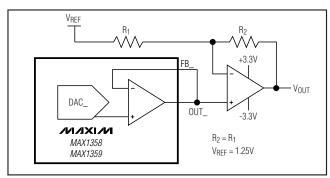
Figure 26. DAC Bipolar Output Circuit
