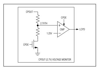
Figure 10. CPOUT Voltage-Supervisor Block Diagram
