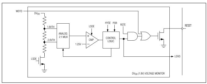
Figure 9. DV<sub>DD</sub> Voltage-Supervisor Block Diagram
