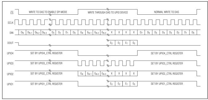
Figure 20. SPI Pass-Through Timing Diagram
