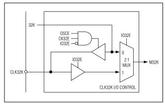
Figure 12. CLK32K I/O Block Diagram
