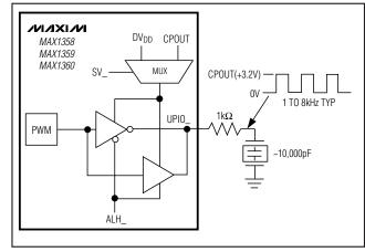
Figure 36. Single-Ended Piezoelectric Buzzer Drive
