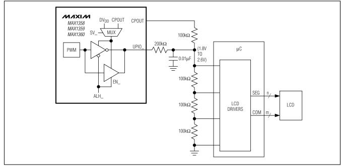
Figure 33. LCD Contrast-Adjustment Application
