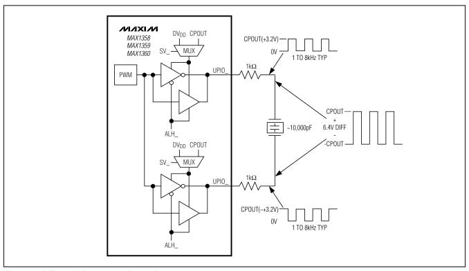
Figure 37. Differential Piezoelectric Buzzer Drive
