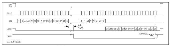
Figure 18. Performing an ADC Conversion (DRDY Function can be Accessed at UPIO Pins)
