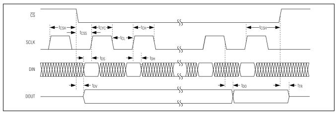
Figure 1. Detailed Serial-Interface Timing
