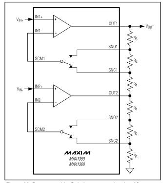
Figure 32. Programmable-Gain Instrumentation Amplifier
