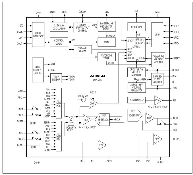
Figure 4. MAX1359 Functional Diagram
