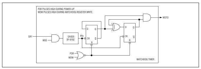
Figure 13. Watchdog Timer Block Diagram
